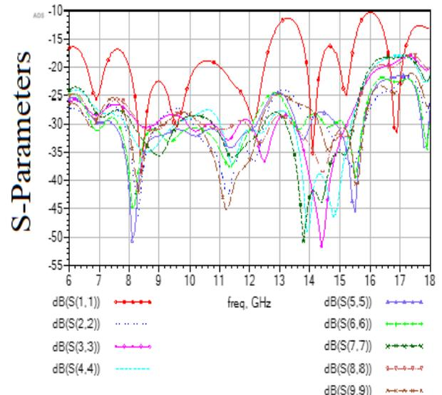
Fig. 6: Return Loss of Multi-Section 8-Way WPD.
