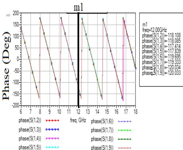
Fig. 9: Phase of Multi-Section 8-Way WPD.
