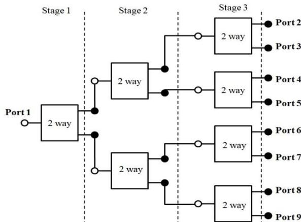
Fig. 3: Multi-Stage WPD Block Diagram.
