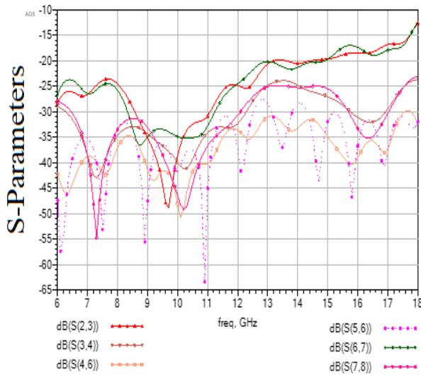
Fig. 7: Isolation of Multi-Section 8-Way WPD.
