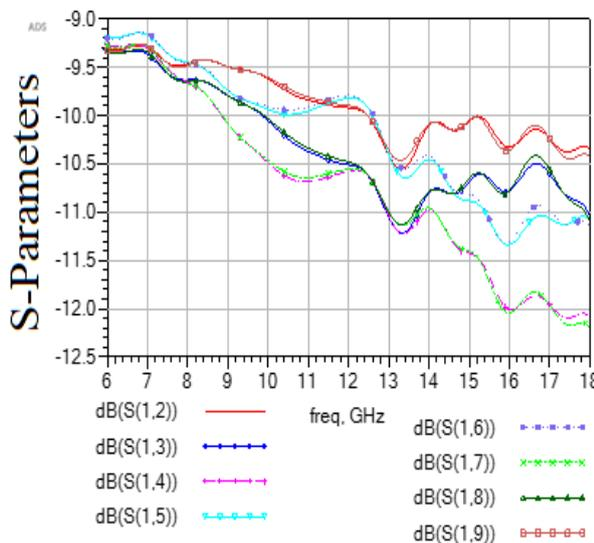
Fig. 8: Insertion Loss of Multi-Section 8-Way WPD.
