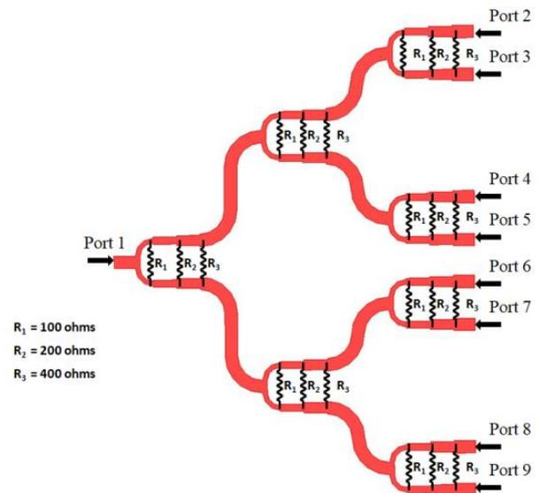
Fig. 5: Layout Diagram of Multi-Section 8-Way WPD.
