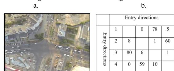
**Fig. 1:** Investigation of a single X-shaped intersection in the city. a. Image of the investigated intersection; b. The result of the study of the traffic intensity through the intersection in the form of OD matrix
