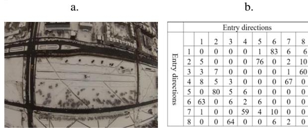
**Fig. 2:** Investigation of a group of X-shaped intersections in the city. a. Image of the group of intersections; b. The result of the study of the traffic intensity through the group of intersections in the form of OD matrix
