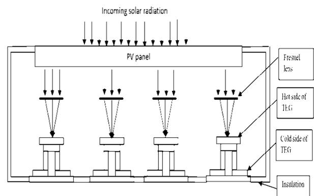
Fig. 6: PV-TE Indirectly Coupled PV-TE System.
