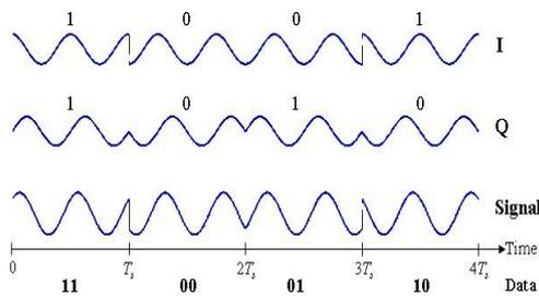
Fig. 6: QPSK Waveform
