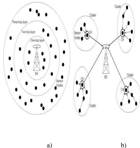
**Fig. 1:** Wireless sensor network architecture: a) layered architecture, b) clustered architecture. (BS: Base Station, CH: Cluster-Head)
