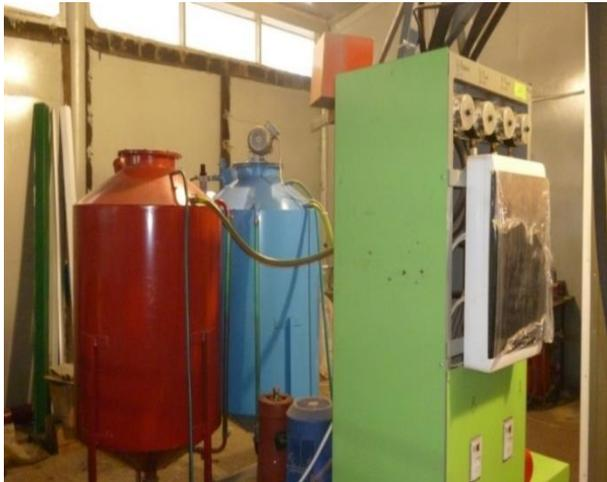
Fig. 8: The equipment for Manufacturing Filled Polyurethane Foam.
