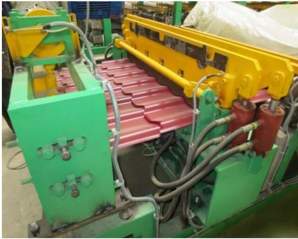
Fig. 7: The technology of manufacturing "Monterrey" Tiles.
