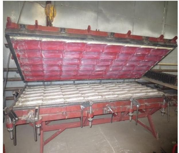
Fig. 10: Clay Plate Mould.
