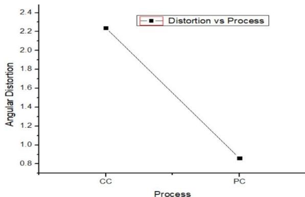
Fig. 8: Effect of Weld Process Distortion.
