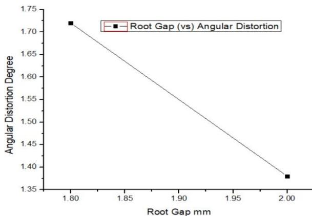
Fig. 7: Effect of Root Gap on Distortion.
