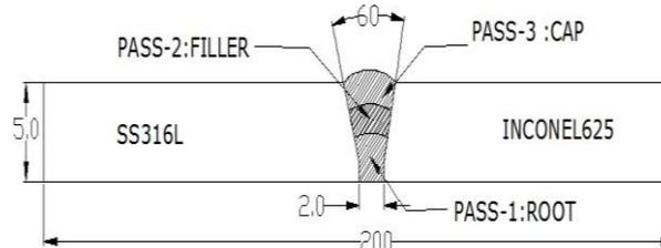
Fig. 1: GTA Welded Samples.
