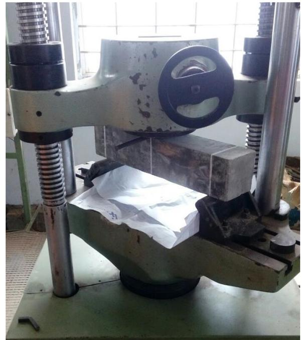
Fig.8: Universal testing machine
