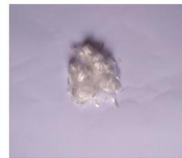
Fig.6: Polypropylene fibre
