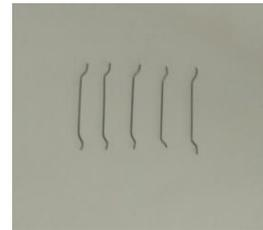
Fig.5 Steel fibre
