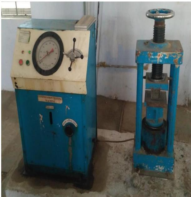
Fig.7: Compression testing machine
