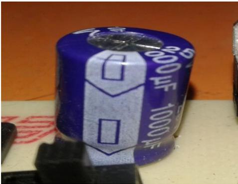
**Fig. 5:** Capacitor Filter Used in the Power Supply Module.
