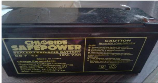
Fig. 10: Storage Battery Used in the Smart Uninterrupted Power Supply System.
