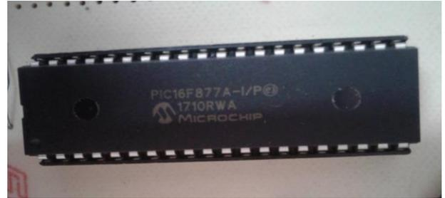
**Fig. 7:** Microcontroller Used in the Smart Uninterrupted Power Supply System.
