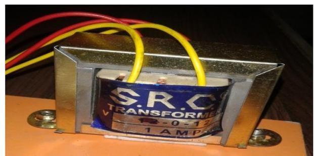
**Fig. 3:** Transformer Used in the Power Supply Module. Rectifier is used to convert AC to DC, and this process is known as rectification. The bridge type full wave rectifier is used in this paper and it is depicted in Figure 4.
