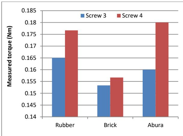
Fig. 3: Measured Torques for Same Screw Types with Different Head Types.
