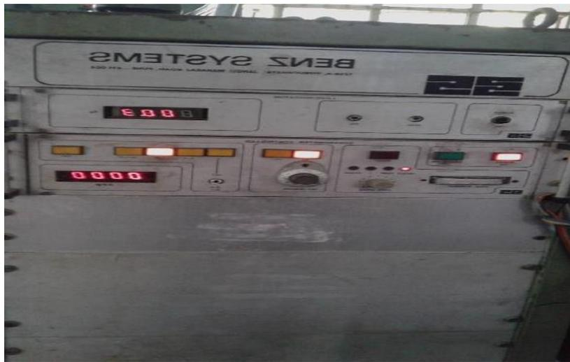
Fig. 5: Digital Load Controller
