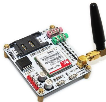
Fig. 7: GSM Modem
