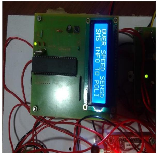
Fig. (g): Over speed control mode
