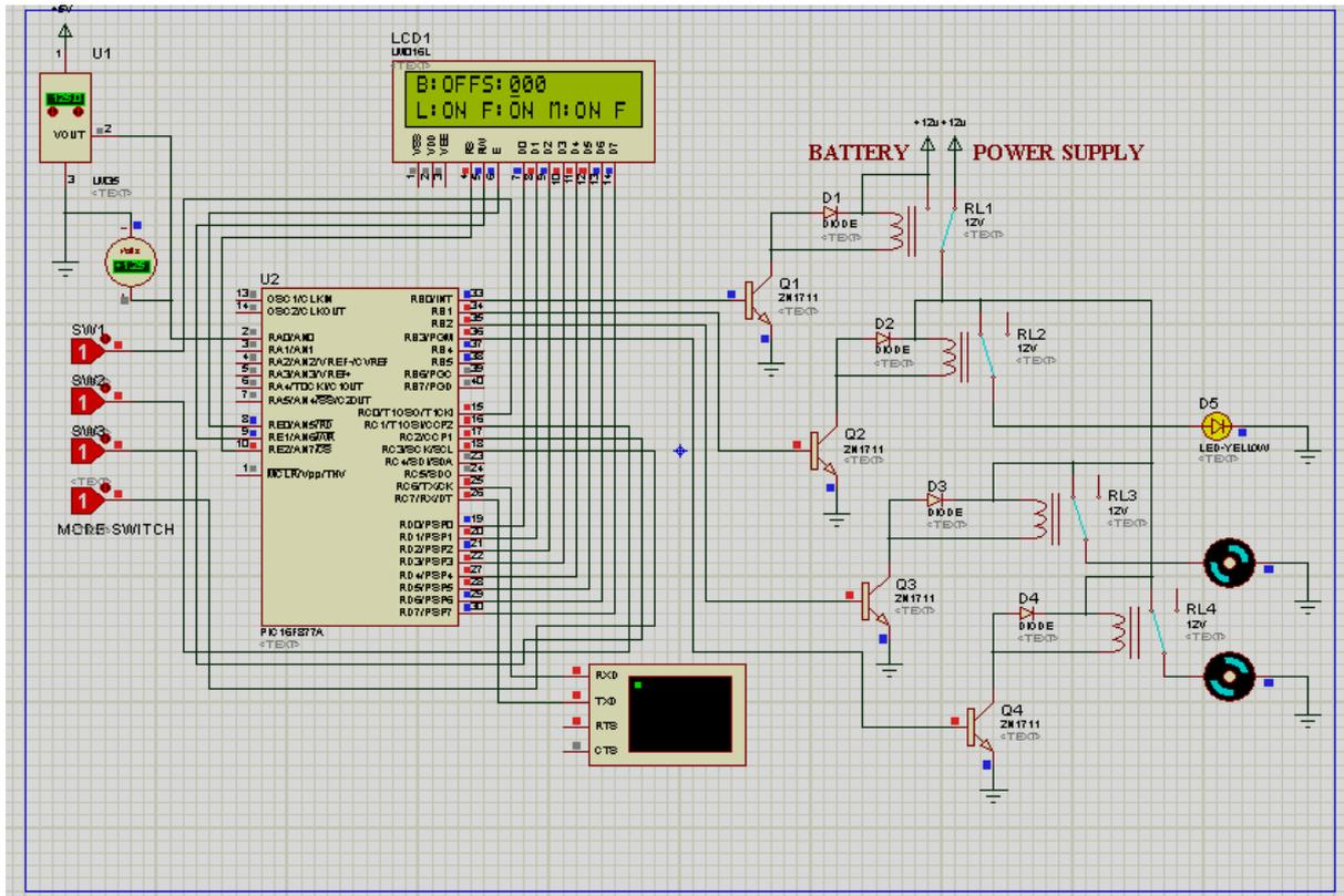
Fig. 4: Simulation During Power Supply Mode
