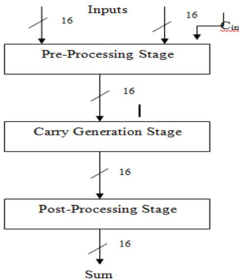
Fig. 2.3: Structure of Brent-Kung adder
