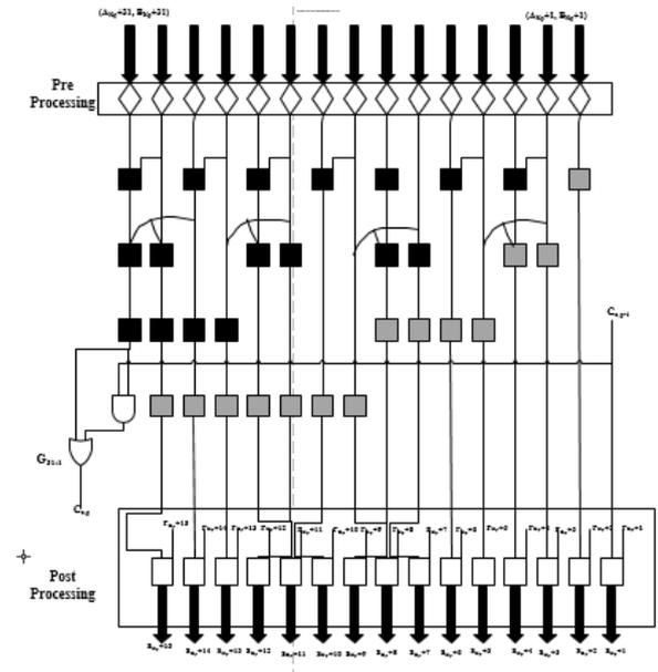
Fig. 2.7 Internal structure of Sklansky cska
