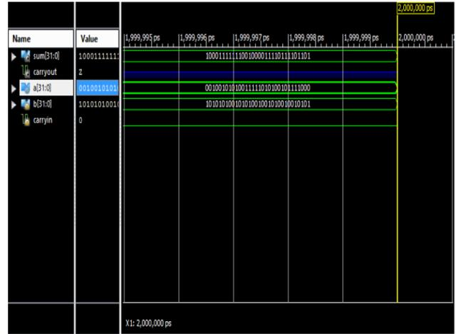
Fig. 3.1: Output wave form of CSKA's
