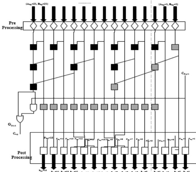
Fig. 2.2: Internal structure of Brent Kung cska
