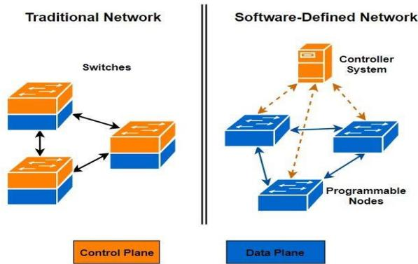
Fig. 1: Comparison between Traditional and SDN networks
