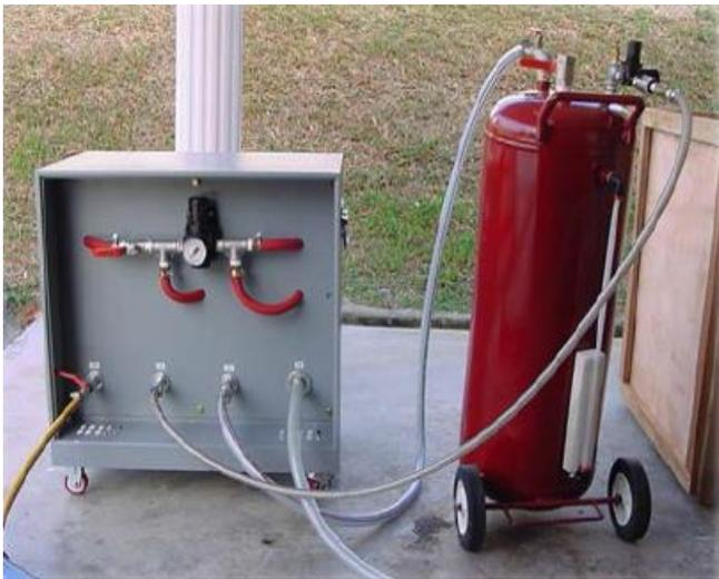
Fig. 3: Foam generator TM1
