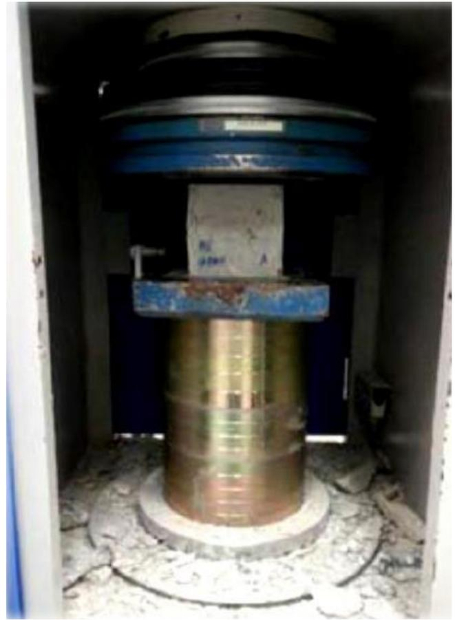
Fig. 4: Compression test on HPC cube
