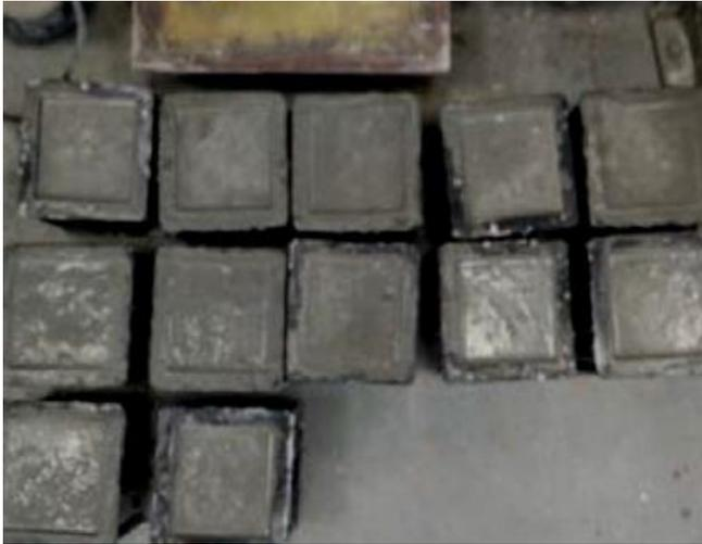
Fig. 2: Cube samples prepared for this study
