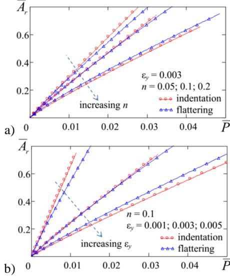
**Fig. 1.** Dependencies  $\bar{A}_r - \bar{P}$  for different values of hardening parameters.
