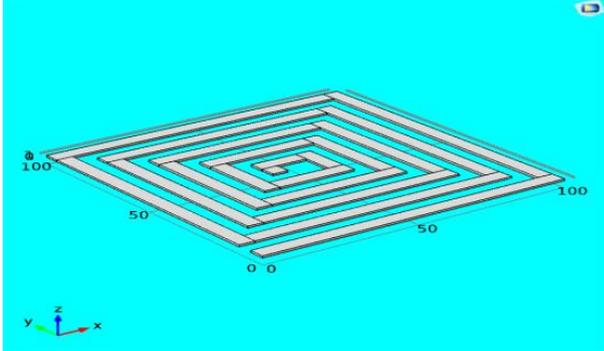
Fig. 1: Spiral cantilever structure
