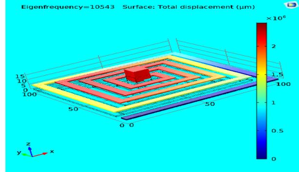
Fig. 2: Frequency analysis of 20 beam structure
