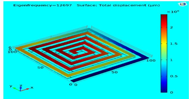
Fig. 3: Simulation of 20 beam structure with tip mass
