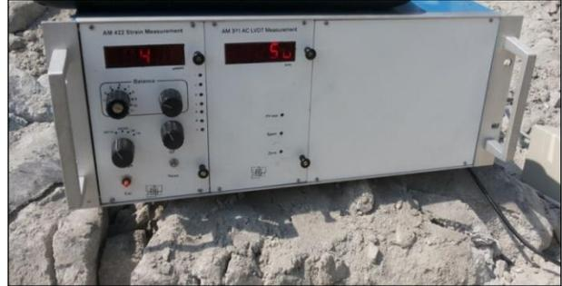
Fig. 12: Conventional data logger with display unit in the field
