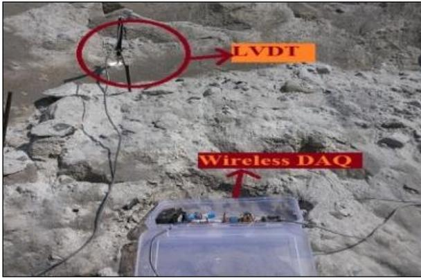
Fig. 10: Installation of sensors during field studies
