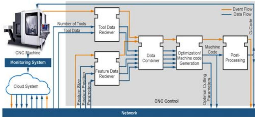
Fig.5: Cloud Architecture of CNC Simulator
