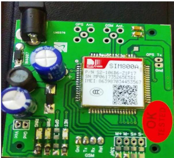
Figure 2: GSM Module (SIM800A)
