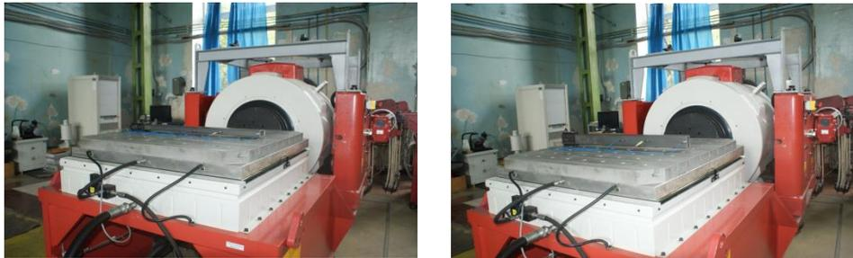
**Figure 3.** The samples mounted on a vibrating table.
