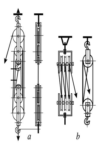
Fig. 8. Multi-pass pulley blocks (6 ручьев): a – pulleys in on plane
