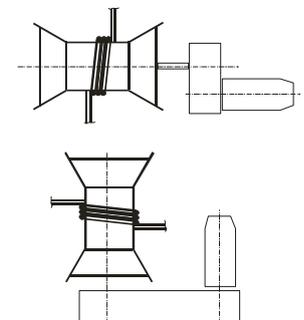
Fig. 33. Electric capstan winch with horizontal and vertical drum position
