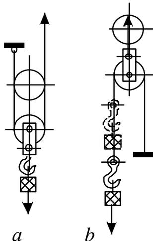
Fig. 7. Both single-pass: a – with forth enhance, b – with speed and distance enhance
