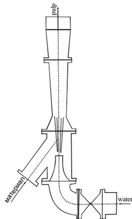
Fig. 43. Hydro elevator
