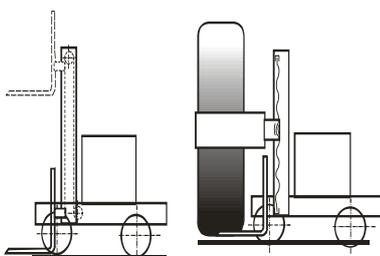
Fig. 13. Chain hoist in the electric stacker
