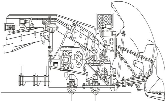
Fig. 34. Loader PPN, back discharging
