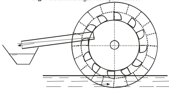
Fig. 45. Rotary water lifter
