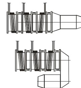
Fig. 32. Scraper three-drum hoist with co-axis and parallel engine position
