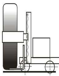
Fig. 14. Screw jack in the wheels lifter
