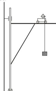
Fig. 17. Bracket crane with variable boom
