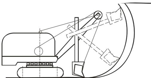
Fig. 36. Straight scoop excavator
