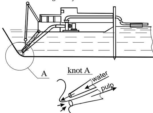
Fig. 44. Bucket dredger with hydrowashout
