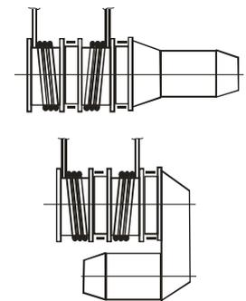
Fig. 31. Double-drum hoist with co-axis and parallel engine position
