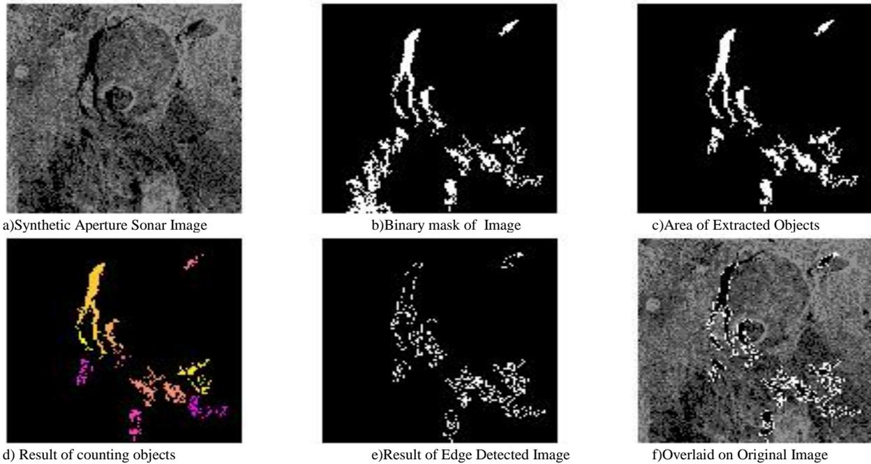
Fig.2. SAR Image after Segmentation operation using proposed Hybrid PSO Method
