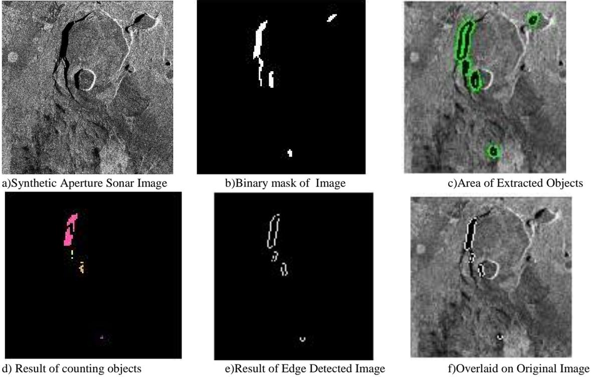
Fig.1. SAR Image after Segmentation operation by Hybrid region based active contour method
