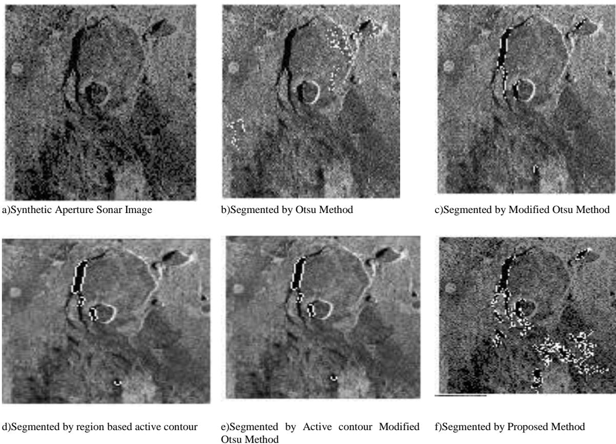
Fig. 3: SAR Image after segmentation operation using various techniques.
