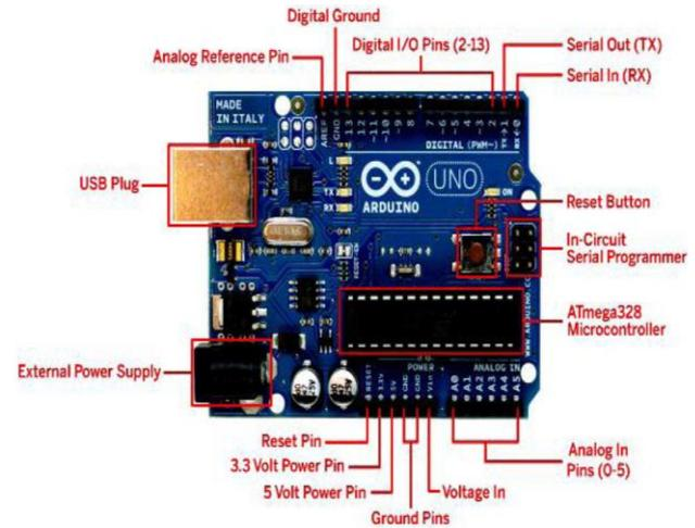
Fig. 3: Arduino UNO Board Sources: <https://www.Arduino.Cc>.
