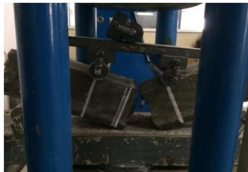
Fig-7b. Sisal fiber Concrete after testing
