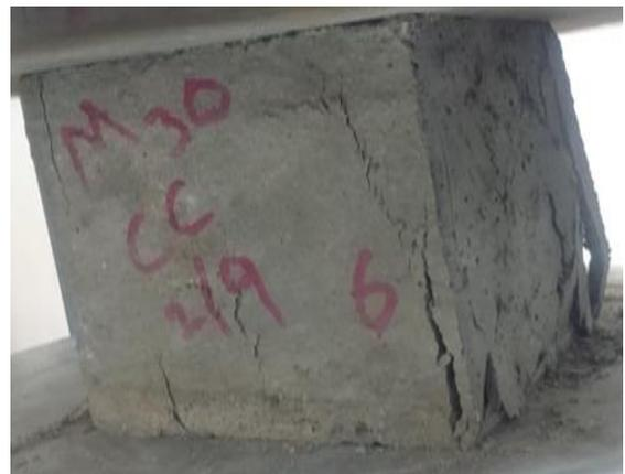
Fig-4b. Conventional Concrete after testing
