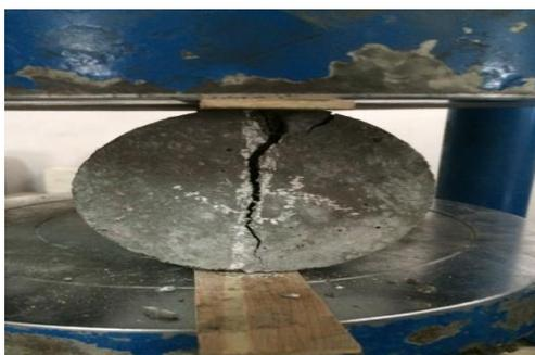
Fig-6b. Sisal fiber Concrete after testing
