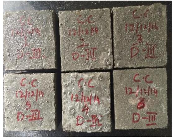
Fig-4a. Conventional Concrete before testing
