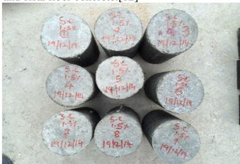
Fig-6a. Sisal fiber Concrete before testing
