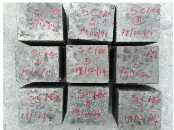
Fig-5a. Sisal fiber Concrete before testing
