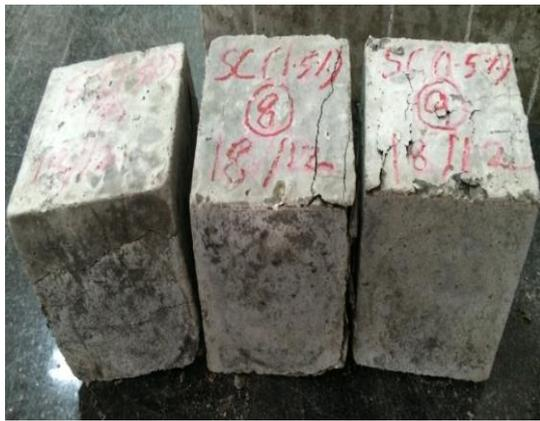
Fig-5b. Sisal fiber Concrete after testing
