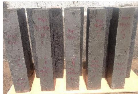
Fig-7a. Sisal fiber Concrete before testing
