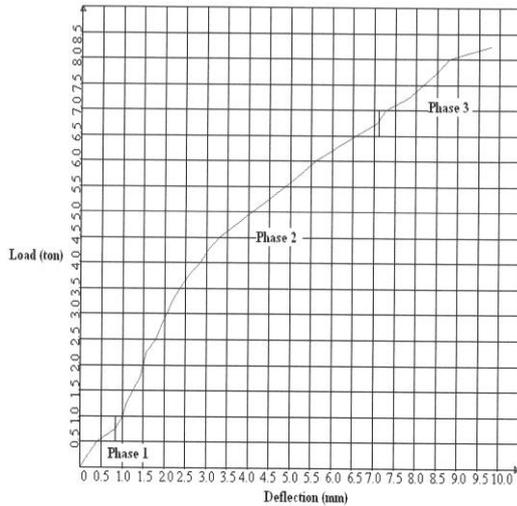
Fig 5 Load deflection curve for solid slab
