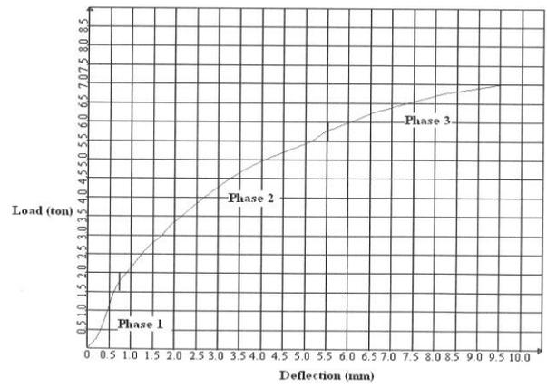
i) Load deflection curve for slab with 2.28% voids
