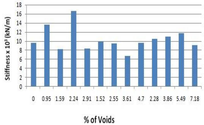
**Fig 8** Stiffness to Percentage of voids in Phase 2
