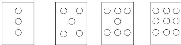
Fig 2 Laying of balls in Line, X, I and Matrix configuration
