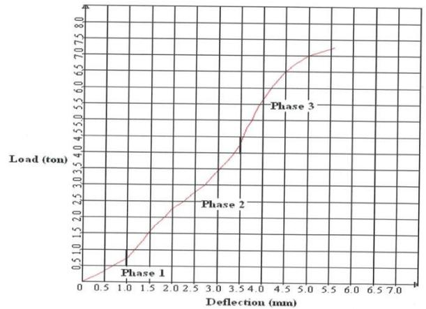
k) Load deflection curve for slab with 5.49% voids
