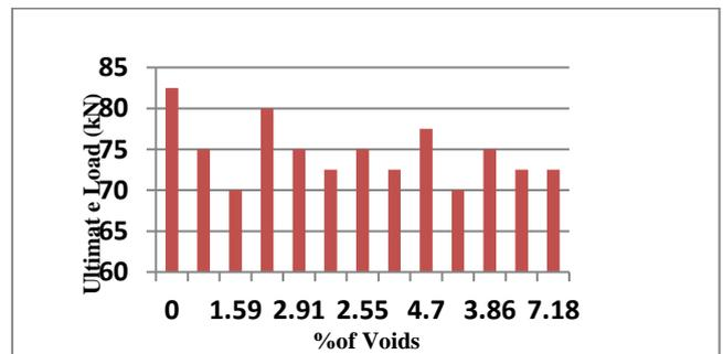
Fig 4 Variation of Ultimate load to % of voids
