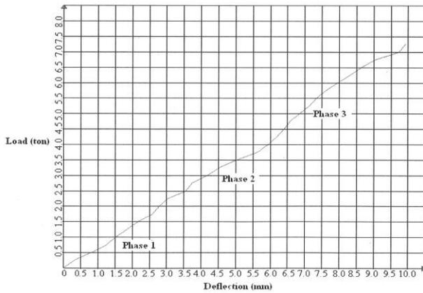
g) Load deflection curve for slab with 3.61% voids
