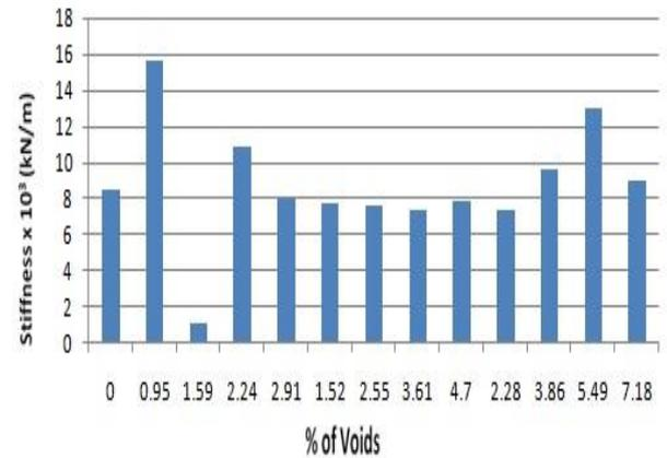
**Fig 9** Stiffness to Percentage of voids in Phase 3
