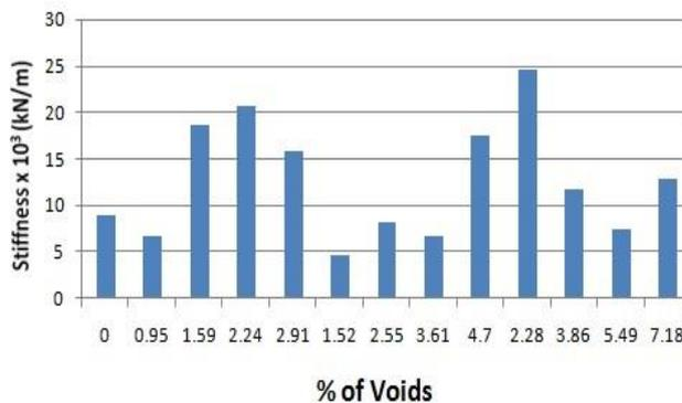
**Fig 7** Stiffness to Percentage of voids in Phase 1
