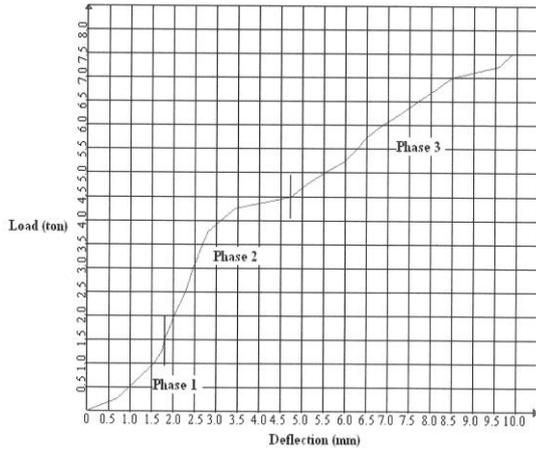
e) Load deflection curve for slab with 1.52% voids
