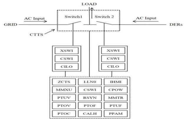
**Fig. 2:** CTTS Mapping to IEC 61850.
