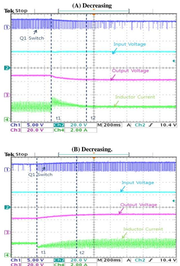
Fig. 9: Input Voltage Fluctuation Characteristics increase.
