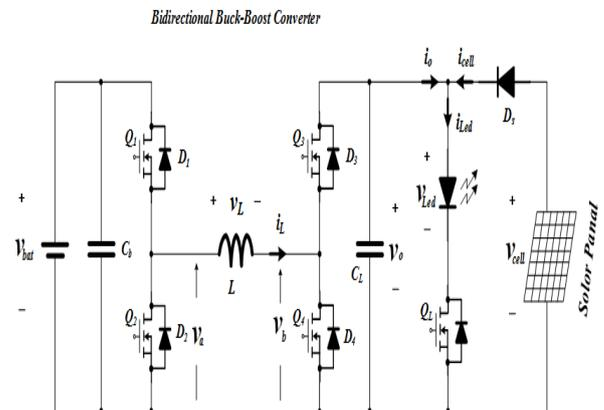
Fig. 3: Proposed DC / DC Converter System.
