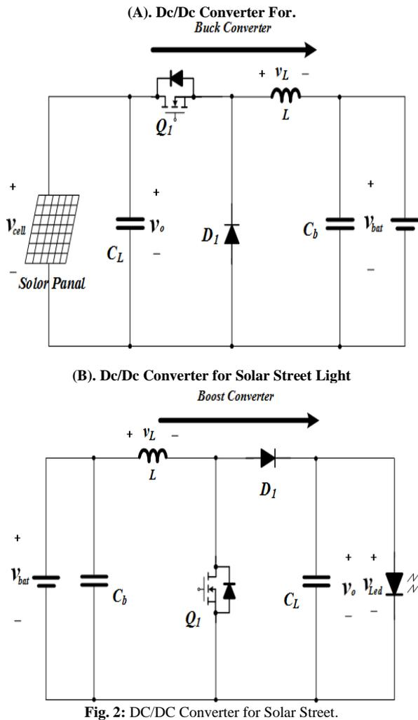
Fig. 2: DC/DC Converter for Solar Street.
