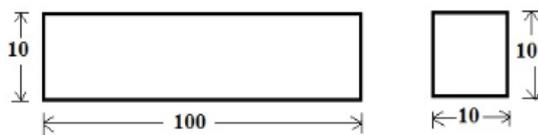
**Fig. 5:** Dimensions of the Specimen as Per ASTM D790 for Three-Point Bend Test.
