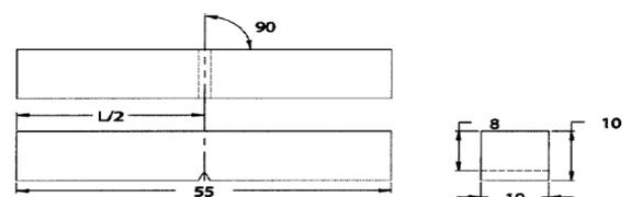
**Fig. 3:** Cross-Sectional Views of Specimen as Per ASTM E23 Standards for Impact Test.
