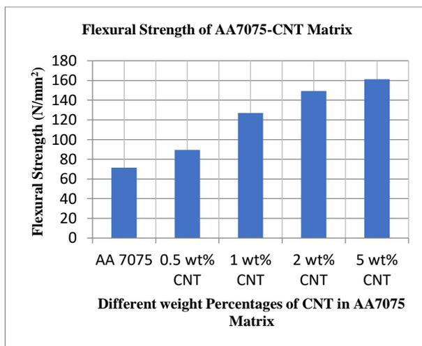
**Fig. 6:** Variation of Flexural Strength of AA7075-CNT Matrix with Increase in Weight Percentage of MWCNT.
