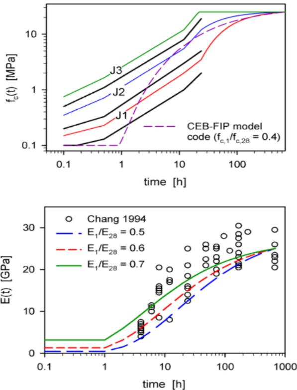
Fig. 1: Evaluation of Shotcrete Strength and Stiffness with Time [17].
