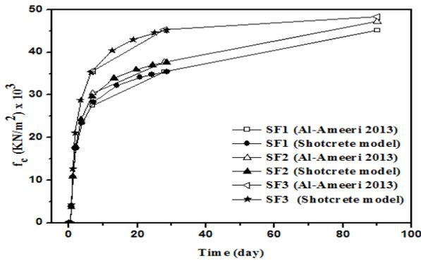
Fig. 5: Shotcrete Model Validation for Concrete Compressive Strength Development with Time.
