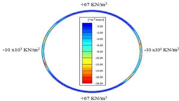
Fig. 6: Principal Compression and Tensile Stresses along the Tunnel Lining.
