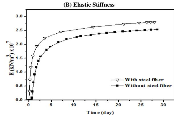
Fig. 12: Development of Compressive Strength and Elastic Stiffness of Reinforced and Unreinforced Tunnel Lining with Time.
