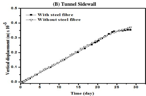
Fig. 15: Effect of Steel Fibre Content on the Development of Lining Displacement with Time.
