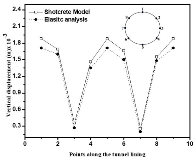
Fig. 18: Vertical Displacement along the Tunnel Lining Using the Shotcrete Model and the Elastic Analysis.
