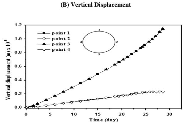
Fig. 7: Development of the Stress and Vertical Displacement around the Tunnel Lining With Time.
