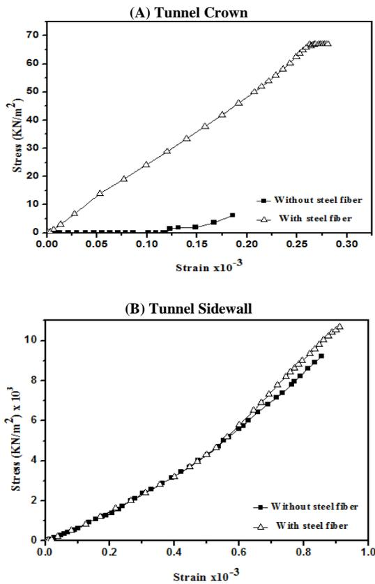
Fig. 14: Stress-Strain Curve of the Reinforced and Unreinforced Tunnel Lining.
