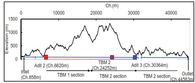
Fig. 3: Cross Section of Pahang-Selangor Water Transfer Tunnel.
