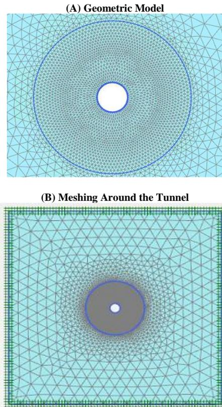
Fig. 4: A) Geometric Model, B) Mesh around the Tunnel.
