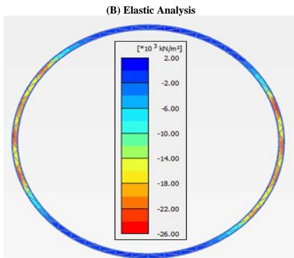
Fig. 16: Distribution of Major Principal Stress of the Tunnel Lining Using (A) Shotcrete Model and (B) Elastic Analysis.
