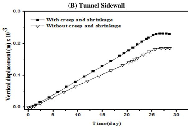
Fig. 11: Effect of Creep and Shrinkage Strain on Development of Lining Displacement with Time.
