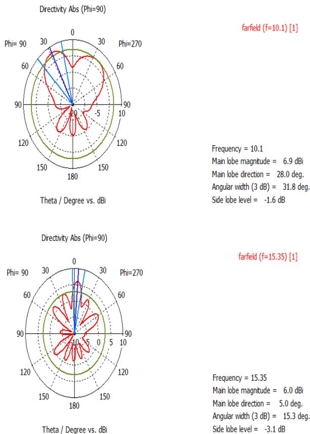
Fig. 3: Polar Plot of Antenna at 10.1 GHz And 15.35GHz.
