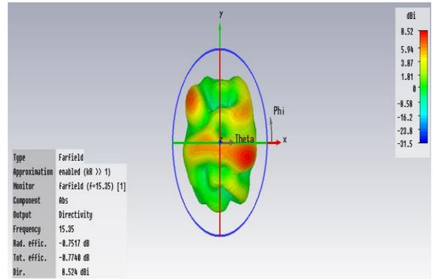
Fig.4: 3D Pattern of Presented Antenna at 10.1 GHz and 15.35 GHz.
