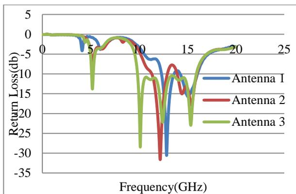
Fig. 6: Return Loss vs. Frequency of Antenna1, Antenna2 and Antenna3.
