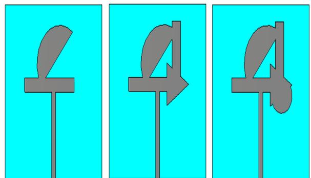
Fig. 5: Geometry of the Proposed Antennas (A) Antenna1 (B) Antenna2 (C) Antenna3.
