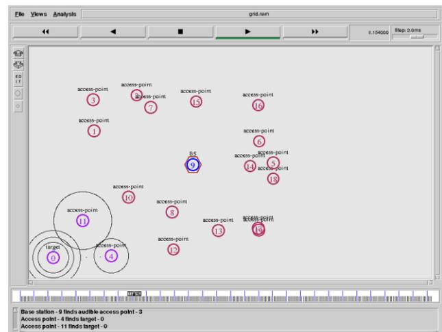
**Fig 4.5** The one Access Point among those N number of the AP's near the Target node are set as temporary base station to identify the location of the Target node.
