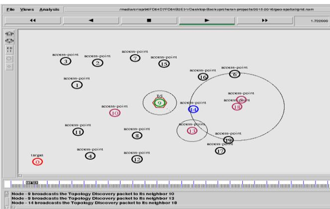
**Fig 4.2** The base station tries to establish connection among the n number of the APs.
