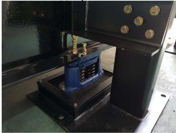
Fig. 2: Passive-Type Mount Module for Electric Power Plant.
