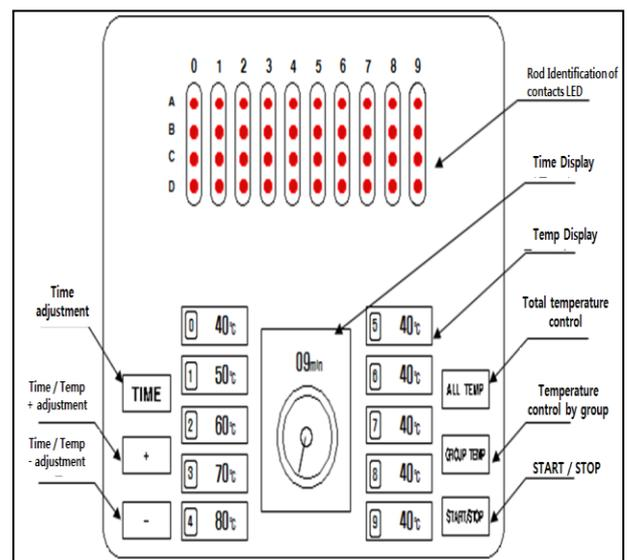
Fig. 3: Screen Configuration of Display Part.
