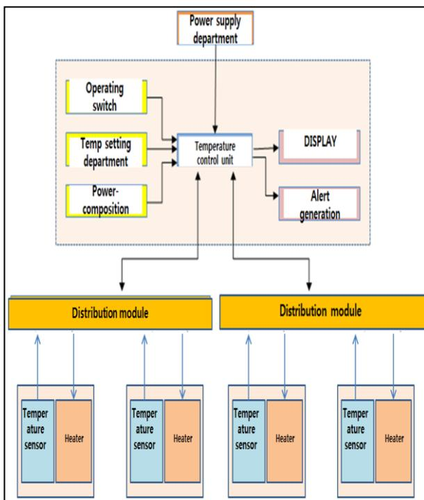
Fig. 1: Block Diagram of Control Board in Digital Perm Equipment.
