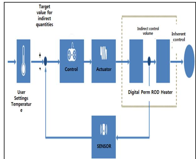
Fig. 2: Block Diagram of Temperature Control Circuit.
