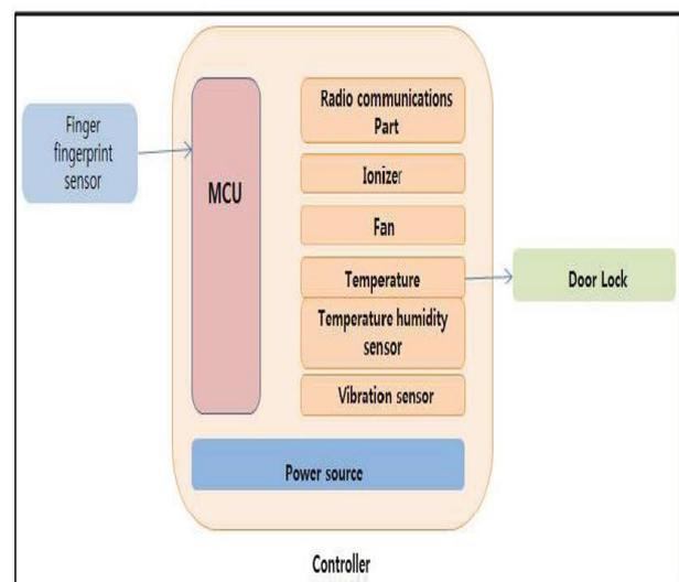
Fig. 1: Control Unit Block Diagram in Furniture Based on Iot Device.
