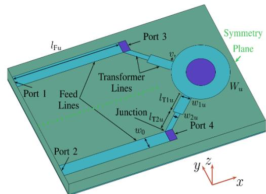
FIG 1: Diagram representation of single element in circular patch.
