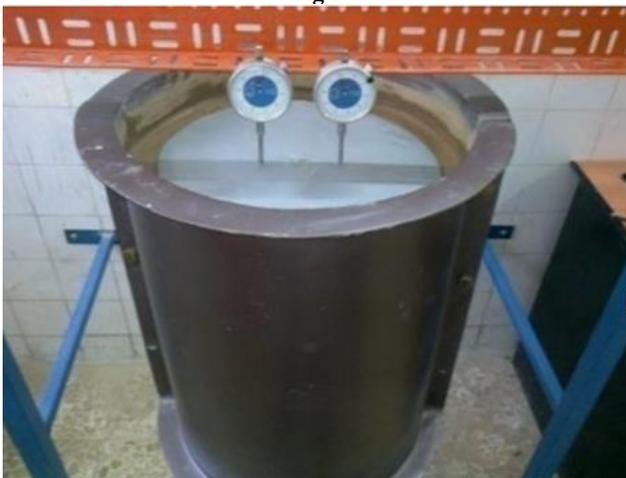
Fig.2 Plate of (GPA-Foundation system) under the heave
