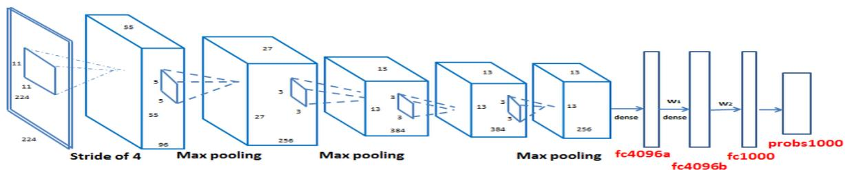
Fig. 4: AlexNet Architecture
