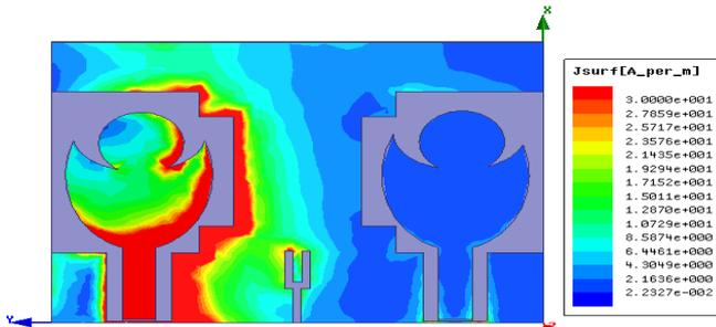
Fig. 5 (a): Current distribution at 3.1 GHz.
