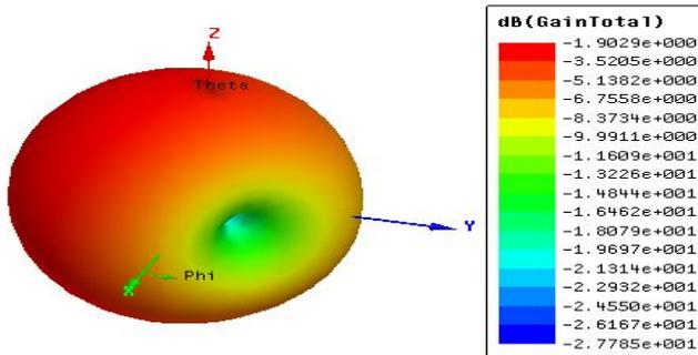
Fig. 8 (b): 3-D polar plot at 5.6 GHz.
