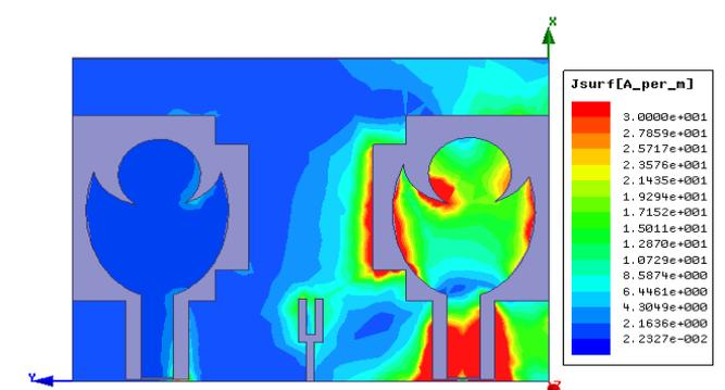
Fig. 6 (c): Current distribution at 10.6 GHz.
