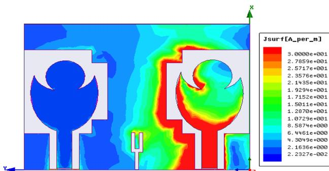
Fig. 6 (a): Current distribution at 3.1 GHz.
