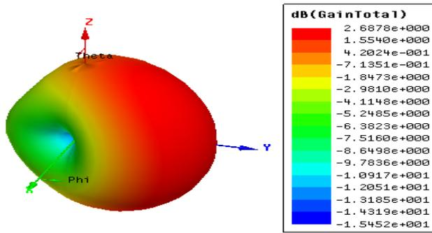
Fig. 7 (c): 3-D polar plot at 10.6 GHz.
