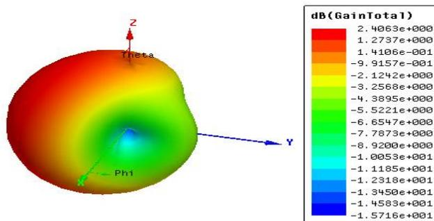
Fig. 8 (c): 3-D polar plot at 10.6 GHz
