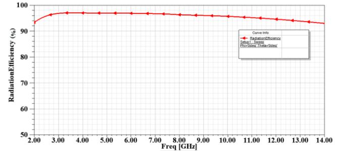
Fig. 11: Radiation efficiency of the simulated antenna.
