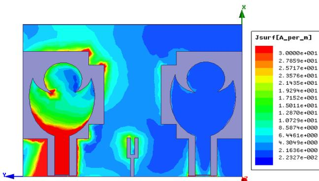
Fig. 5 (b): Current distribution at 5.6 GHz.
