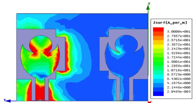
**Fig. 4 (b):** With T stub and without Y slot on ground.
