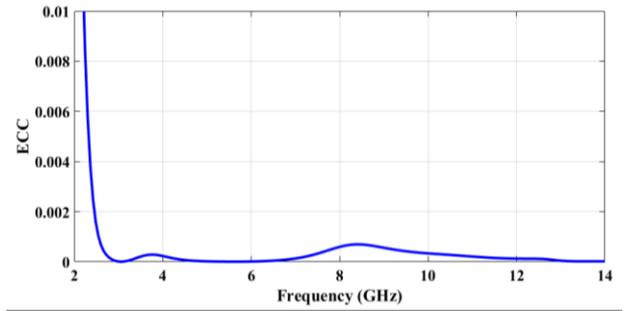
Fig. 9: ECC of the simulated antenna
