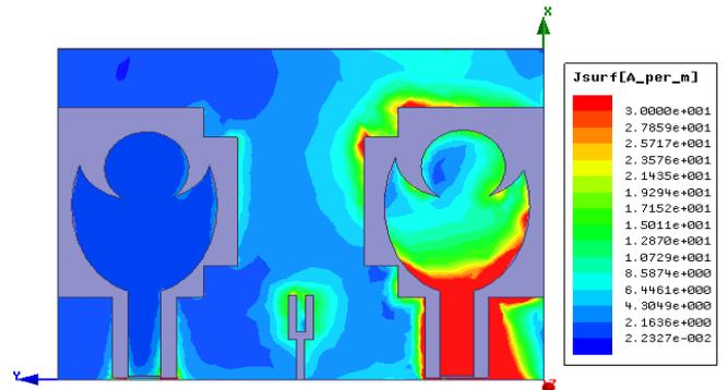
Fig. 6 (b): Current distribution at 5.6 GHz.
