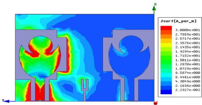
Fig. 5(c): Current distribution at 10.6 GHz.
