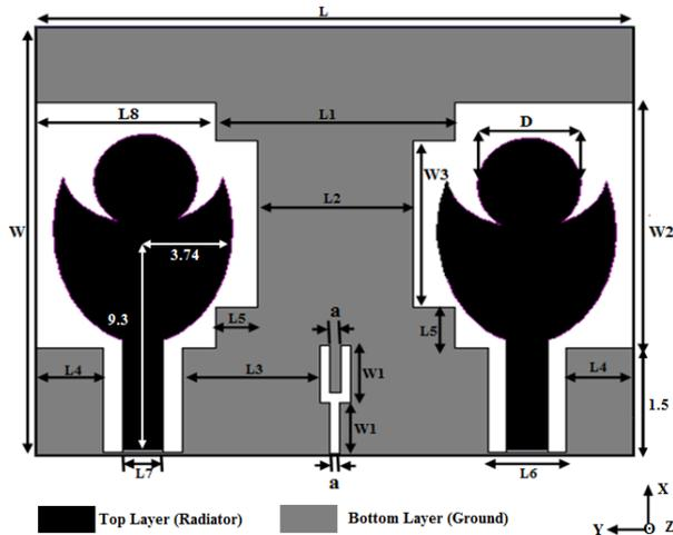
**Fig. 1:** Geometry of the proposed UWB MIMO antenna
