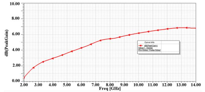
Fig. 10: Peak gain of the simulated antenna.
