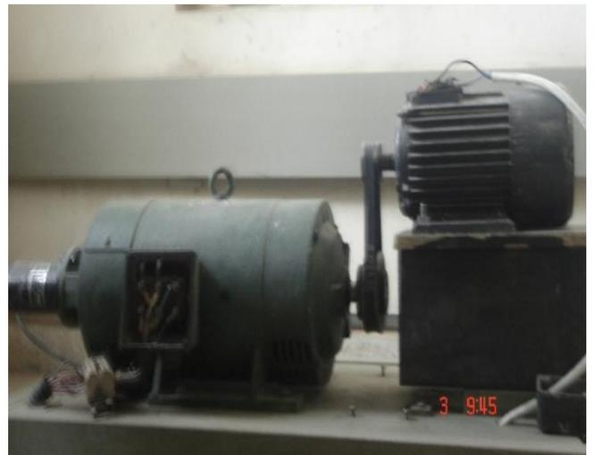
Fig. 5: Flexible Coupling
