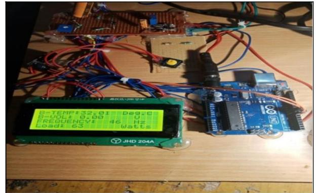
Fig. 7: Parameter Monitoring of Ups Remotely with IoT.
