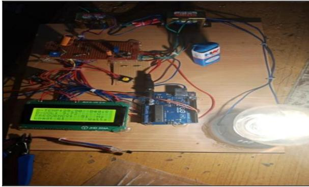
Fig. 3: Shows the Implementation of the Monitoring of the UPS Under the Load Conditions.
