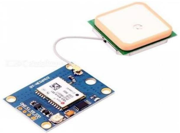
Fig. 3: Picture of GPS Module.
