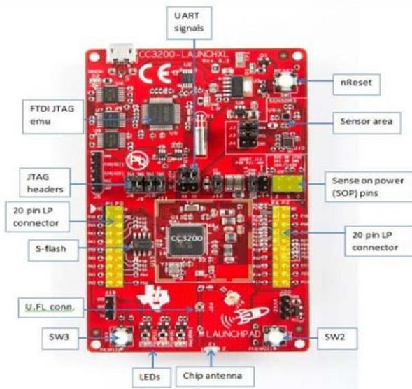
Fig. 1: TI CC3220S Hardware KIT.
