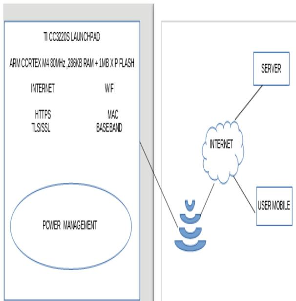
Fig. 4: Working Prototype.
