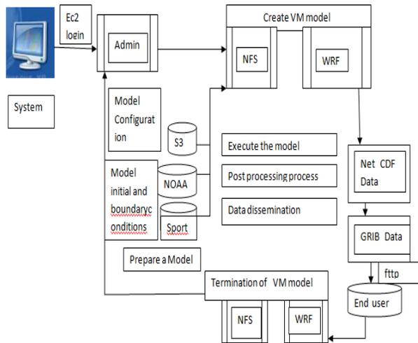
**Fig. 3:** Weather Forecasting Model by Using Cloud Computing Techniques [5].
