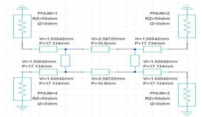
**Fig 2.** Schematic of proposed quadrature patch hybrid coupler: w=width of the Microstrip, p=length of the Microstrip
