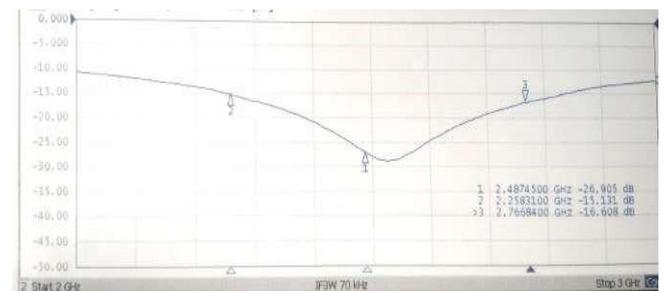
Fig 10. Isolation between ports 2 & 3, ports 4& 1
