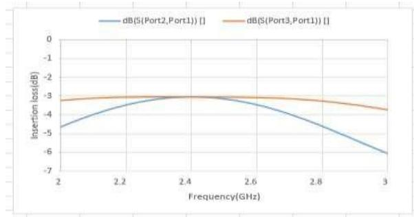
Fig 5. Insertion loss at port 2 and port 3
