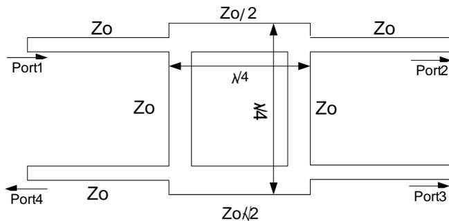
**Fig1.** Structure of quadrature hybrid coupler:  $Z_0$ = impedance of free space,  $\lambda$ =Operating Wave Length
