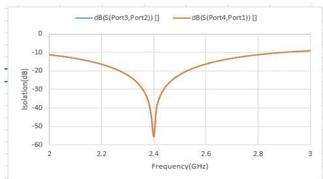
Fig 7. Isolation between ports 2 &3, ports 4& 1
