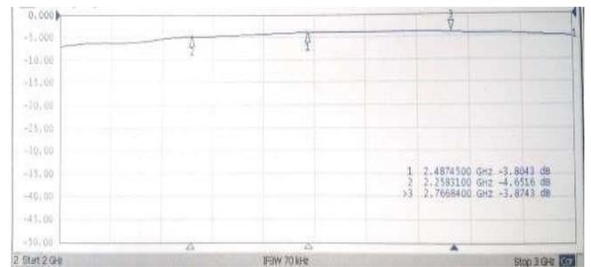
Fig 9. Insertion loss at port 2 and port 3
