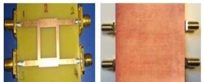
**Fig 4.** Fabricated patch hybrid front view and back view
