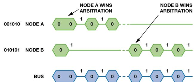
Fig. 6: The arbitration logic between two nodes [9]
