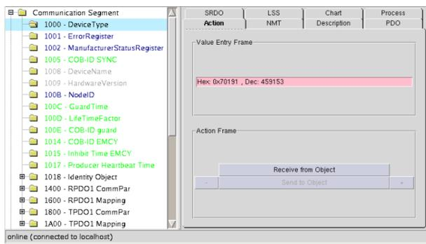
Fig. 11: The CANopen Device monitor (CDM)
