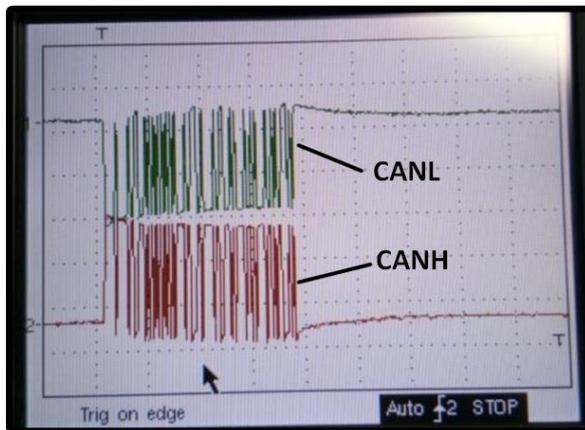
Fig. 12: A message sent between node 1 and gateway node
