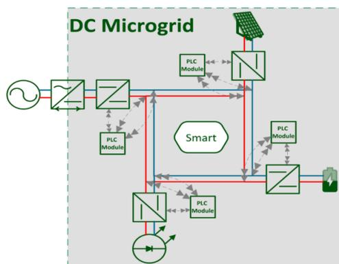
Fig. 1: A mesh DC micro grid
