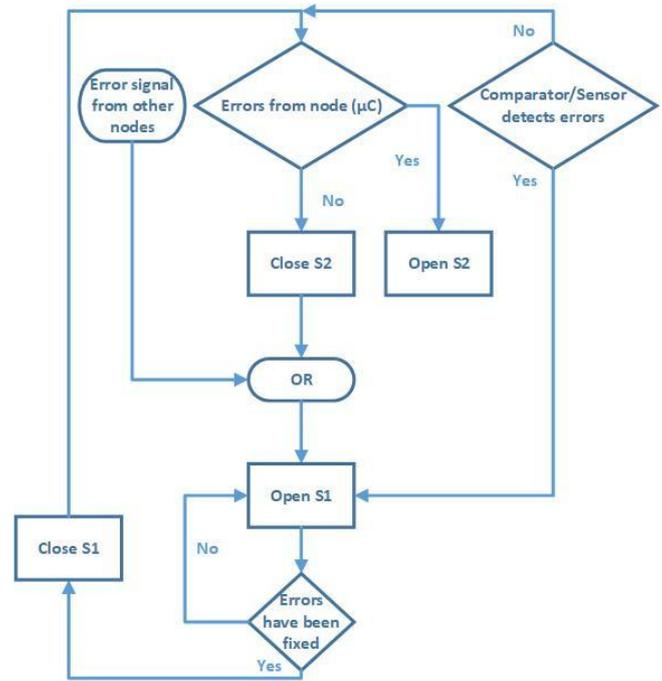
Fig. 9: Operation of the self-protection system
