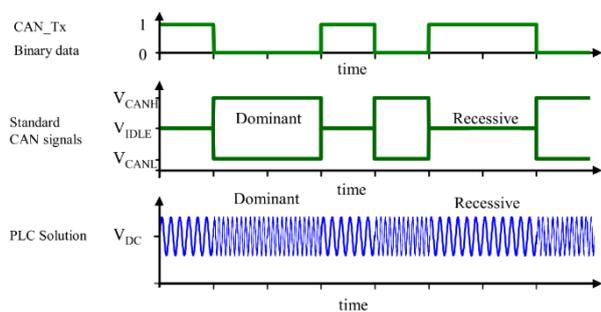
Fig. 4: Comparison between the standard CAN and the modulation of PLC evaluation based on FPGA board to implement CAN bus over PLC. FPGA will be shrunk in an ASIC next month [6].
