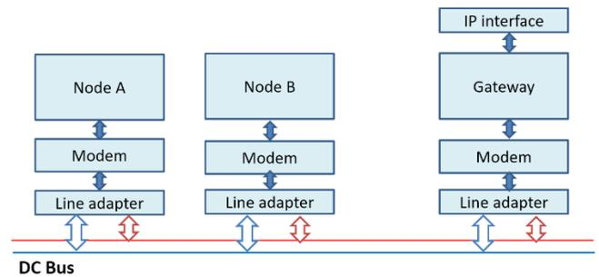
Fig. 5: A PLC solution on DC bus
