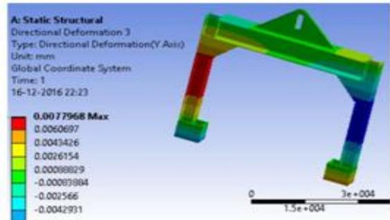
Fig. 6: Total deformation of the structure
