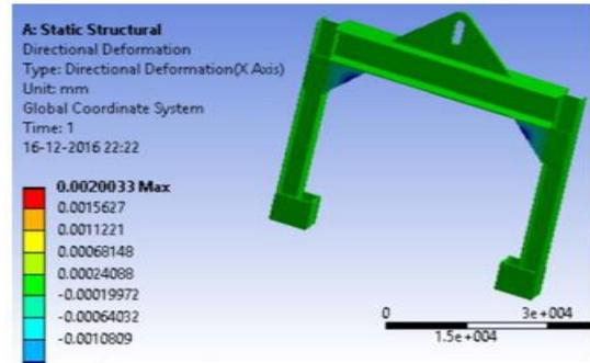
Fig. 7: Directional deformation in X axis
