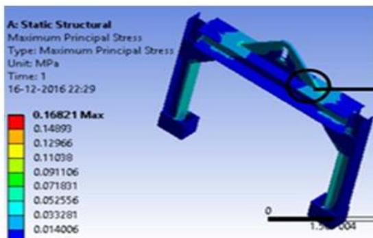
Fig. 9: Maximum Principle Stress
