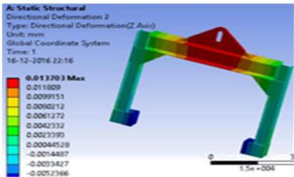
Fig. 5: Directional deformation in Z axis
