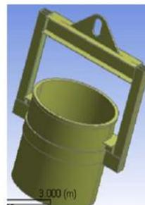
Figure 1 CAD Model of crucible structure
