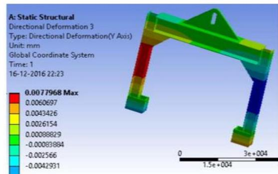
Fig. 8: Directional deformation in Y axis
