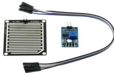
Fig. 4: Rain Drop Sensor
