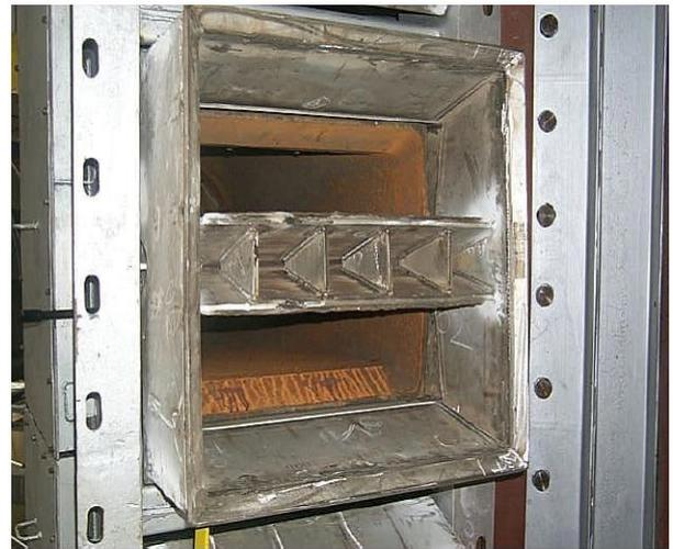
Fig. 2: Burner Nozzle
